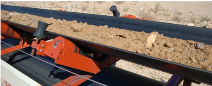
TROUGHING SELF-ALIGNING IDLERS
